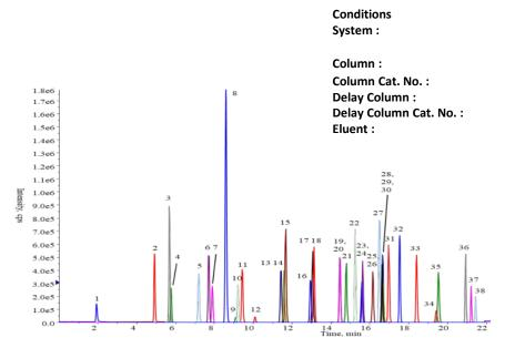
Exion HPLC System (SCIEX) QTRAP 6500+ LC-MS/MS System (SCIEX) InertSustain AQ-C18 (1.9  $\mu$ m, 50 x 2.1mm I.D.) 5020-89938 Delay Column for PFAS (30 x 3.0 mm I.D.) 5020-90005 A) CH<sub>3</sub>OH B) 20 mmol/L CH<sub>3</sub>COONH<sub>4</sub> in H<sub>2</sub>O
